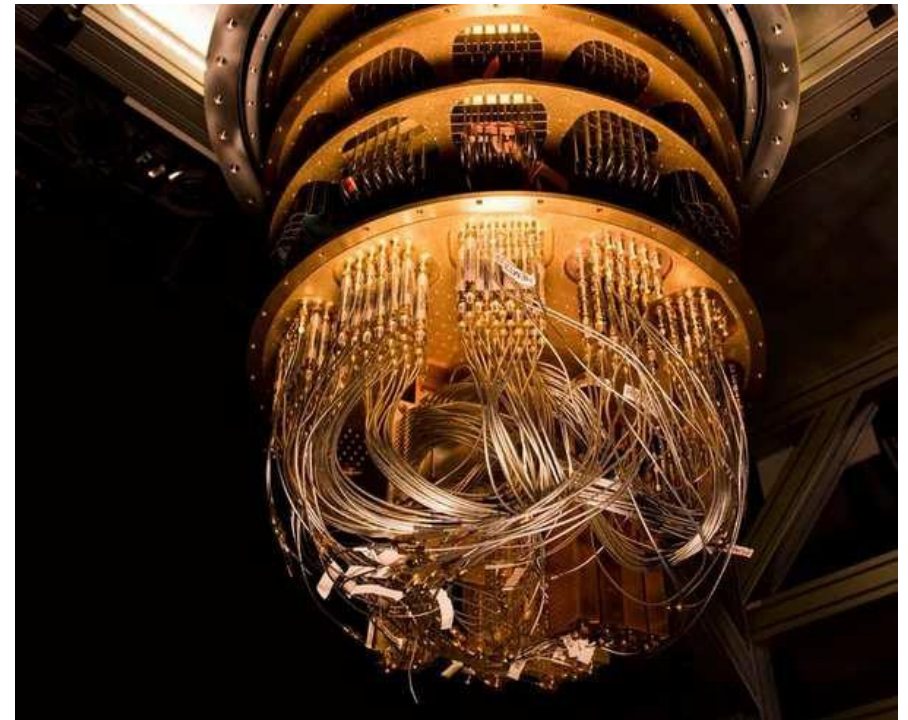
Cryostat of Google's quantum computer. (Google)
